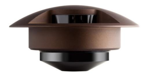
Agena is 70 mm in diameter, 50 mm in length, with a 99 mm ring. An accurate passive heat sink technology and an operating temperature electronic control guarantee that the luminaire will last in time with an ambient temperature up to +60°C.
