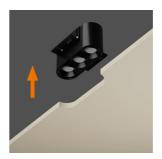
MAINTENANCE Remove luminaire by pulling the M3 screws
