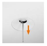
MAINTENANCE ASYMMETRICAL Remove luminaire by pulling the suction cup
