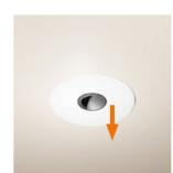
MAINTENANCE SYMMETRICAL Remove luminaire by pulling the hex key
