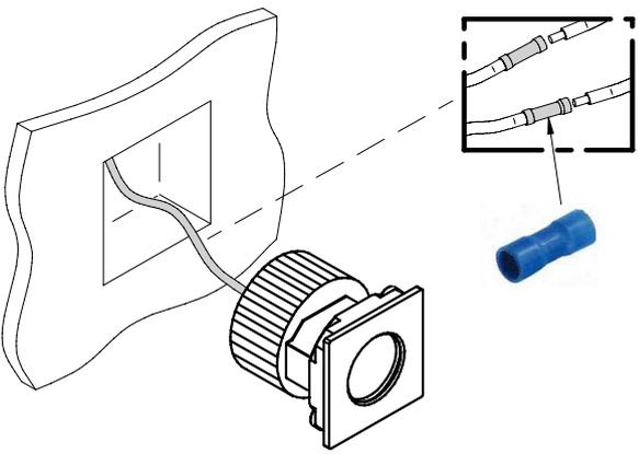
**2** Push the luminaire up to the end and be careful not ruining the inner walls of the housing box. The magnets will hold it in place.
