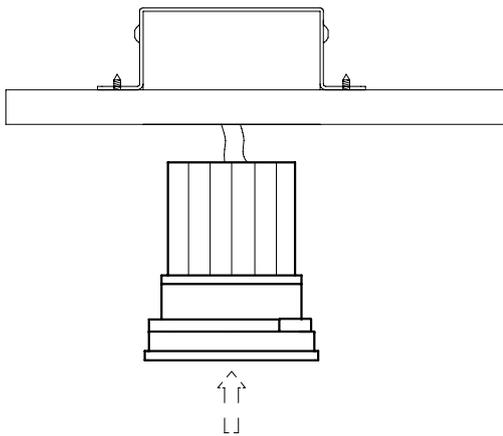
EN: Proper heat dissipation is required when installing the luminaire and, therefore, provide an empty area in the back of the luminaire. Do not sink the luminaire within any materials with low thermal conductivity such as wood, plastic, etc. and do not fix the luminaire with resin, polyurethane foam or silicon.
