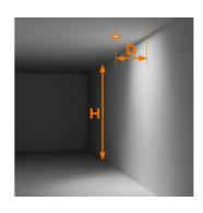
The spacing between luminaires (S) shall be minimum the distance (D) from the wall and maximum twice the distance (D  $\times$  2) from the wall
