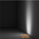
The spacing between **luminaires S** and the distance from the wall D shall be: S, spot  $20^{\circ} = 0.3 \text{ m} / 12^{\circ}$ S, flood  $30^{\circ} = 0.4 \text{ m} / 16^{\circ}$
