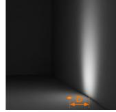
The spacing between **luminaires S** and the distance from the wall D shall be: S, spot  $20^{\circ} = 0.3 \text{ m} / 12^{\circ}$ S, flood  $30^{\circ} = 0.4 \text{ m} / 16^{\circ}$
