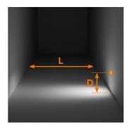
The **spacing between** luminaires (S) and the distance from the floor (D) shall be the same
