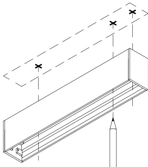
**2** EN: Make the holes, pull out the power supply cable and fix Inserto Medium using the supplied screws.
