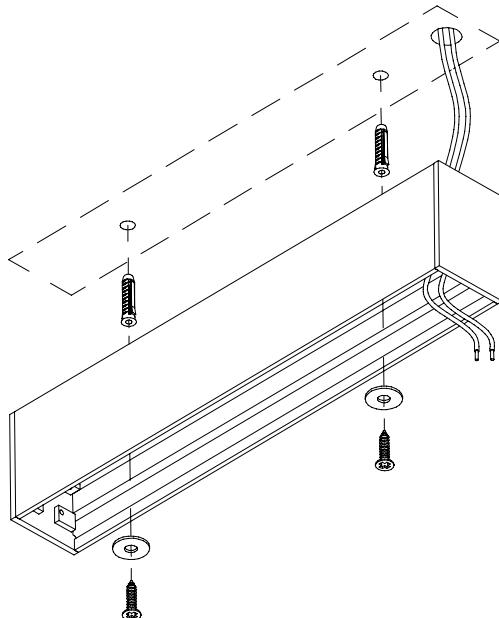
**3** EN: Make the electric connection through the supplied parallelsplices and fix the LED profile pushing it inside Inserto Medium.
