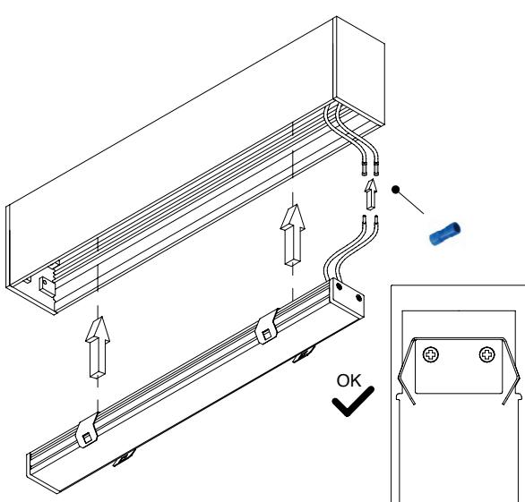
**4** EN: Gently insert the diffuser in the appropriate housing.
